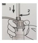
Remove funnel. Place green cap on & turn until the ribs on the cap and cartridge are aligned.
